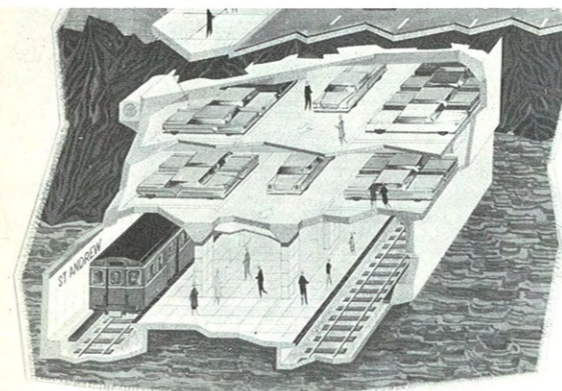
Cut-away view of University Avenue, looking north showing T.T.C. St. Andrew Subway Station with two level garage above.
