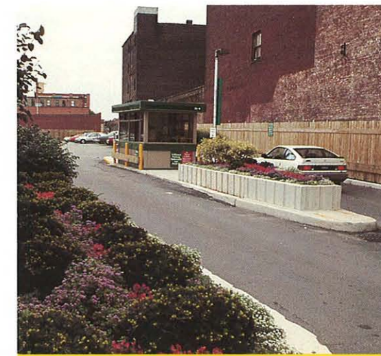
The entrance lane at the Richmond/Sherbourne carpark allows cars waiting to enter the carpark to move in off the road.
